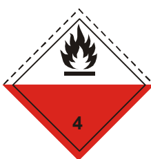
(No. 4.2) Symbol (flame): black; Background: upper half white, lower half red; Figure '4' in bottom corner
